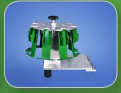
The desired bags and grain count is set via a keyboard. After pressing the start button, the grains are counted and filled continuously.
