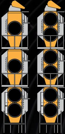
**3400 Series Configuration:** Three modules, four fans & heaters, one on the upper and middle module and two on the lower module. **3Q00 Configuration (Quiet Dryer):** Three modules, three quiet blowers, and four heaters, one on the upper and middle module and two on the lower module.
