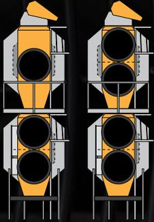
**2300 Series Configuration:** Two modules, three fans and heaters, one on the upper module and two on the lower module. **2Q00 Configuration (Quiet Dryer):** Two modules, two quiet blowers, and three heaters, one on the upper module and two on the lower module.
