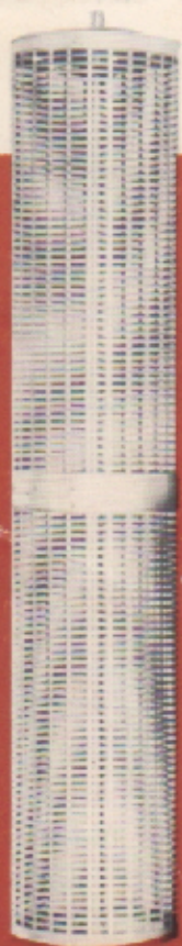
Fig. 4 Cylinder assembly removed and standing on end, which assures thorough clean-out.
